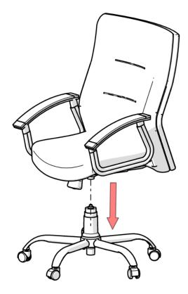
Attach the seat and back assembly of chair to the base assembly (Note: Check the chair to ensure proper fixing) www.hofindia.com
