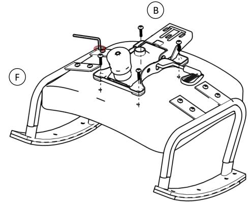
Make sure direction of arrow on mechanism is toward the seat front
