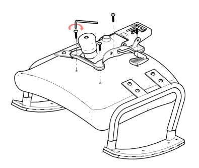
Make sure direction of arrow on mechanism is toward the seat front
