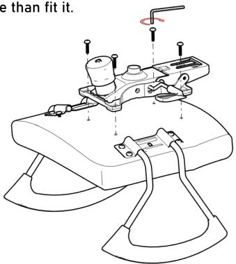
Make sure direction of arrow on mechanism is toward the seat front
