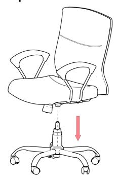
Attach the seat and back assembly of chair to the base assembly
