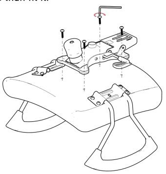
Make sure direction of arrow on mechanism is toward the seat front
