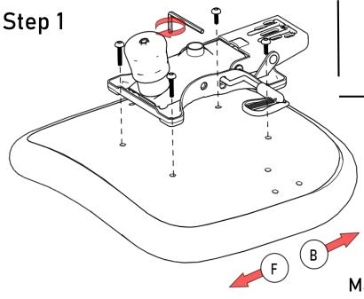
Place seat as shown in image than fit mechanism (Note: focus on right bottom corner annotation F-front B-
