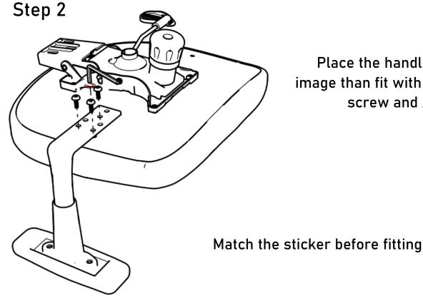
Place the handle as shown in image than fit with the help of Allen screw and Allen key
