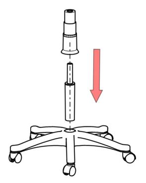
Attach the seat and back assembly of chair to the base assembly
