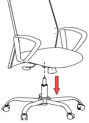
Attach the seat and back assembly of chair to the base assembly
