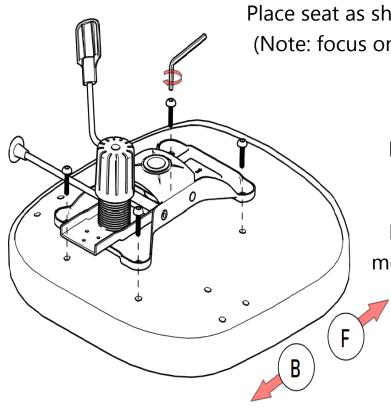
Place seat as shown in image than fit mechanism (Note: focus on right bottom corner annotation **F**-front & **B**-back).
